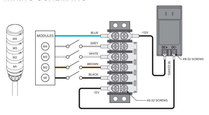
SWITCHES AND CONNECTORS NOT SUPPLIED REFER TO POWER SUPPLY MANUAL FOR MAXIMUM CABLE LENGTH
