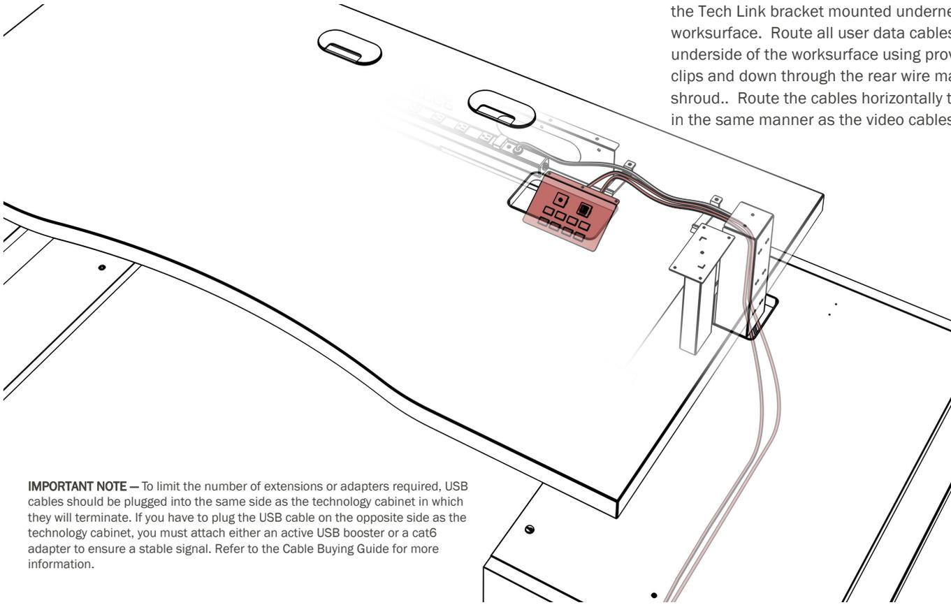
**IMPORTANT NOTE** — To limit the number of extensions or adapters required, USB cables should be plugged into the same side as the technology cabinet in which they will terminate. If you have to plug the USB cable on the opposite side as the technology cabinet, you must attach either an active USB booster or a cat6 adapter to ensure a stable signal. Refer to the Cable Buying Guide for more information.
