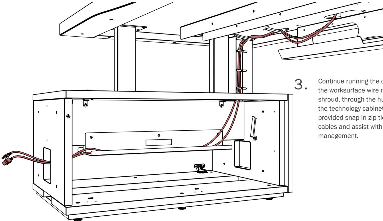
3. Continue running the cables down the worksurface wire management shroud, through the hub, and into the technology cabinets. Utilize provided snap in zip ties to bundle cables and assist with cable management.
